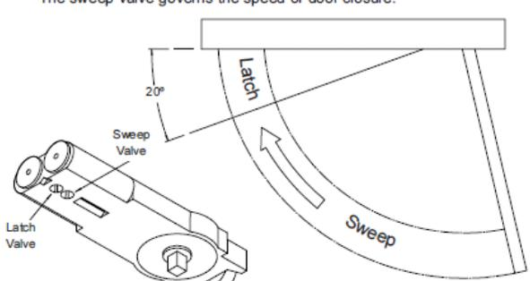
Adjust latch valve by opening door 20° and allowing it to close.
